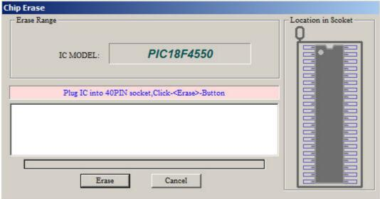
By default, chip ID will be checked before erase. For a small part of the microcontroller, the chip ID cannot be read after encrypted. At that time, don't tick off [check device ID] in the options, otherwise there is an error of checking ID. Click [Erase] button in the dialog box and the erase time will be shown after erase is complete.
