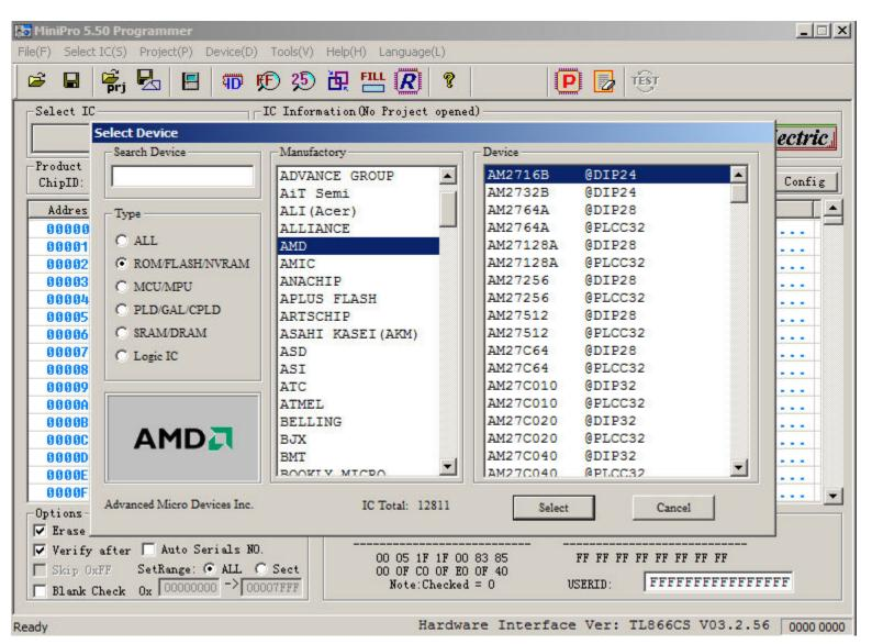
Note: For the IC with same model but different package, if all of the packages (no including DIP package) cannot be listed, you can directly connect the corresponding pins to program by referring to the IC product manual.
