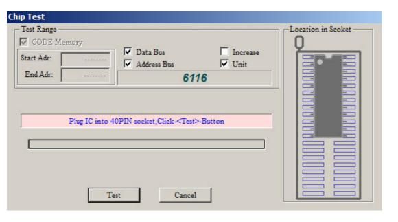
RAM test: There are four methods and the RAM unit can be tested whether the function is normal by these testing methods.
