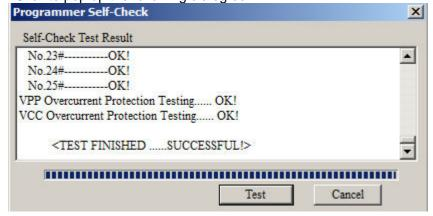
Note: Please remove the IC in the 40-PIN socket and ICSP cable before programmer begins to self-check. The IC may be damaged if no removing. Because when self-checking, programmer will test by applying VPP, VCC and GND to all pins and will perform an inside short-circuit overcurrent test (at the same time apply VPP, VCC and GND to the same pin). The testing information will be shown in the dialog box.
