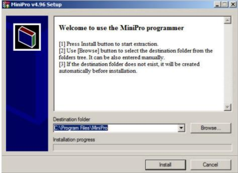
2. The installation progress is quick and the installation of the application will be completed in about 2 seconds. And then the dialog box to install the driver will be popped up automatically, as follows:
