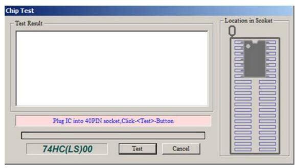
Under normal circumstances, testing information of each logical unit with a variety of input combinations will be shown. If there is an error with IC gate circuit, for example, If you disconnect the PIN1 of 74HC00 chip, the testing results will be shown as follows: prompt chip error.
