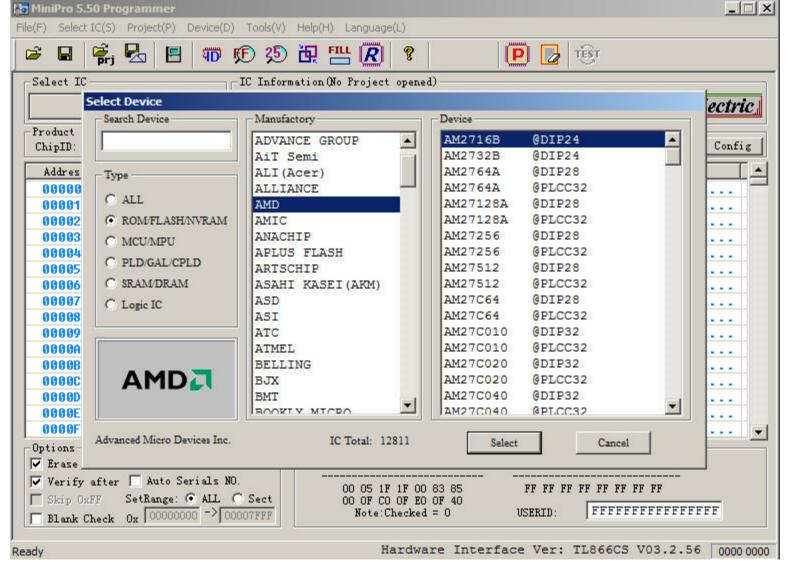
Please note: if some type of packages are not listed in the menu or the present chips are non-DIP packages, you can program by checking the IC product instruction and directly connecting the one-to-one pin.
