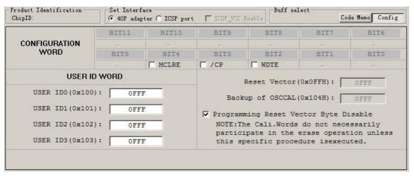
For parts of the PIC chips, by default the programmer will not erase the Reset Vector of the chip when erasing. If you program the verified bytes in configure interface, the Reset Vector will be erased. If the chip has no backup verified value and at the same time you make a mistake with the verified bytes, if you use inside clock, the clock skew may appear and the chip may not be used.
